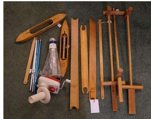
Weaving tools: simple open heddle loom, shuttles, ball winder, niddy-noddy, 100 ml graduated cylinder, and more.
